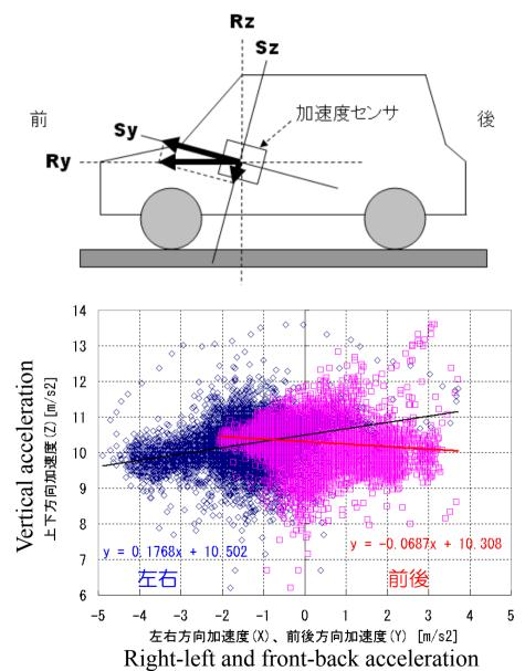
When an accelerometer is tilt, apparent acceleration will be measured on vertical axis at vehicle start, stop, and turn right and left.
