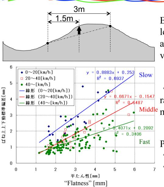
By using sprung moving length, calculate "Flatness" and compared with existing value.
