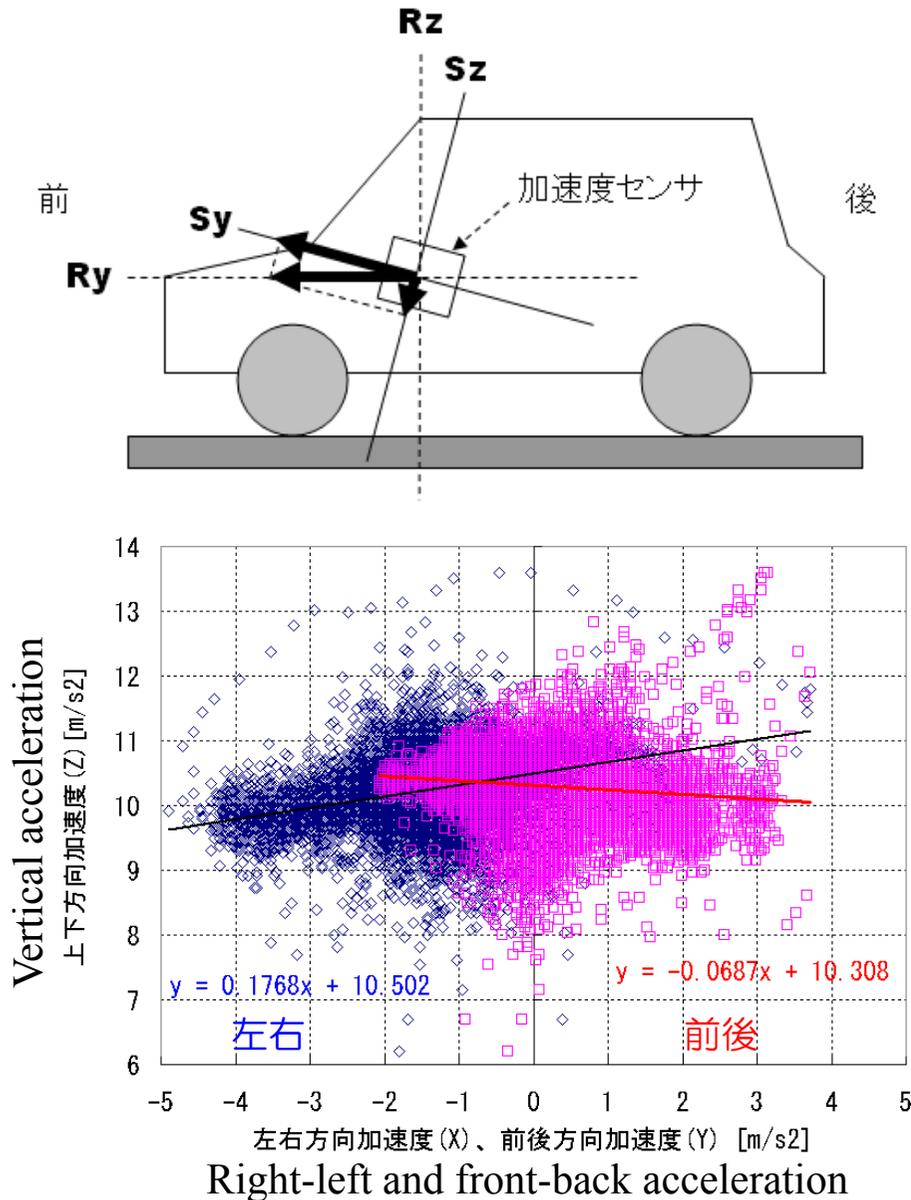
When an accelerometer is tilt, apparent acceleration will be measured on vertical axis at vehicle start, stop, and turn right and left.
